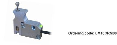
**4) Periodic reference impulse. Every 2 mm.** The LM10 readhead should be ordered with reference mark option C. Magnetic scale should be ordered with **no** reference mark. Position information is output in incremental quadrature format with periodic reference impulses. Reference periods correspond to pole length of magnetisation.
