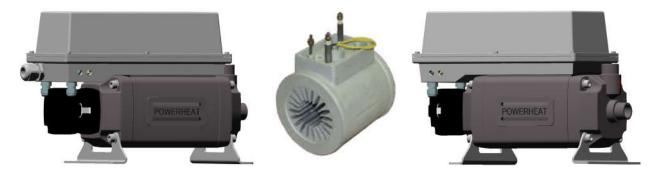
The heat exchanger is based on a die-cast tubular component in aluminum with a large heating surface. The heating element is embedded in aluminum during the die-casting process so therefore completely corrosion proof and not in direct contact with the coolant / liquids. This means a more effective heating and no negative side effects for the coolant / liquids. In addition the Aluminum AS13 is finished with a Teflon coating.
