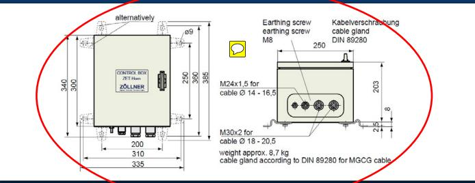
Standard control box (supply voltage 380 / 440 V - control voltage 115 / 220 V) - other voltages on requestions of the control box (supply voltage 380 / 440 V - control voltage  $380 / 440 \text{$
