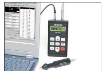
STATWIN 2002 with PC cable and probe RMSQ 0°
