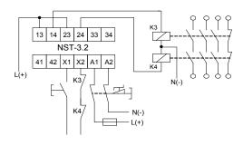
1-channel operation with monitored reset (external contacts)
